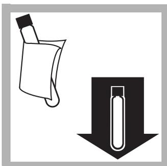
10. Wipe the sample vial and insert it into the 16-mm round cell holder.
