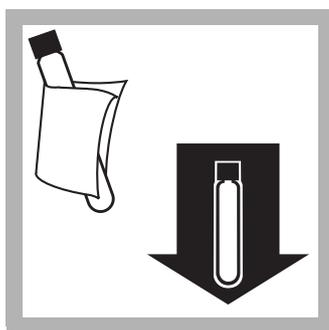
**6.** Wipe the blank and insert it into the 16-mm round cell holder.
