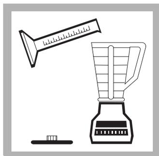
1. Homogenize 100 mL of sample for 30 seconds in a blender. For samples containing large amounts of solids, increase the homogenization time.
